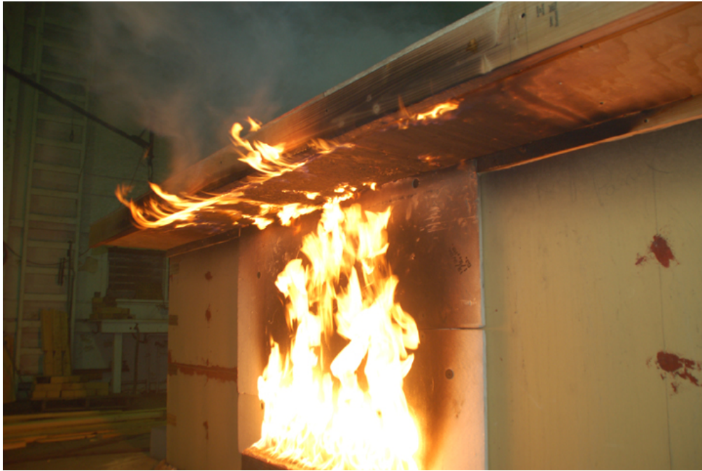
Figure 7. Lateral flame spread was not as extensive in the soffited-eave specimens. In both open- and soffited-eaves specimens, flaming combustion often subsided in charred areas, as shown here. Flaming combustion is more active at the fascia-to-soffit intersection. Flaming in this area was likely enhanced by the addition of a small trim piece that was attached to the soffit material, behind the fascia
