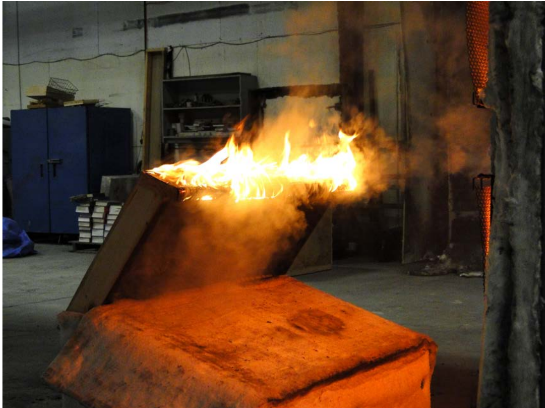
Figure 8. Flaming ignition at the fascia in an open-eave specimen exposed to a 20\text{kW}/\text{m}^2 radiant exposure.
