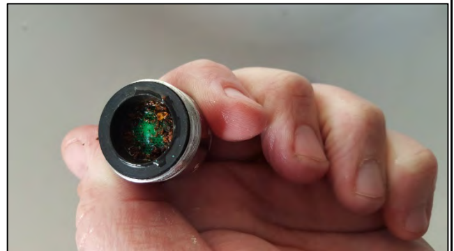
Picture of an aerator with particulate
