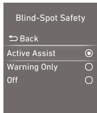
Blind-Spot Collision-Avoidance Assist (BCA) system is designed to help detect and monitor approaching vehicles in the driver's blind spot area and warn the driver of a possible collision with a warning message and audible warning. In addition, if there is a risk of collision when changing lanes or driving forward out of a parking space, the system will help avoid a collision by applying the brake.
