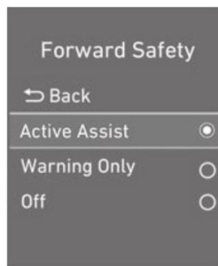
Forward Collision-Avoidance Assist is designed to help detect and monitor the vehicle ahead or help detect a pedestrian or cyclist in the roadway and warn the driver that a collision is imminent with a warning message and an audible warning, and if necessary, apply emergency braking.
