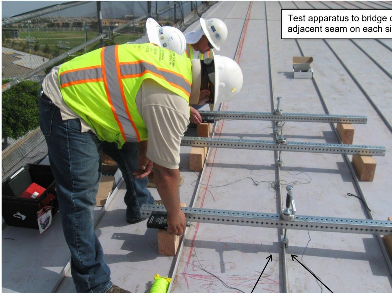
Test apparatus to bridge over adjacent seam on each side.
