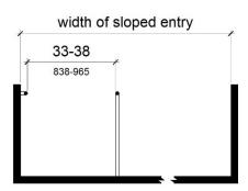
Figure 11B-1009.3.3 Handrails for Sloped Entry
