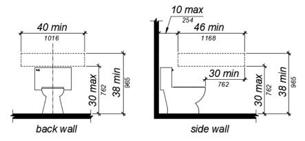
FIGURE 11B-809.10.7.3 REINFORCEMENT FOR GRAB BARS.
