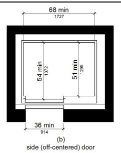
Figure 11B-407.4.1 Elevator Car Dimensions
