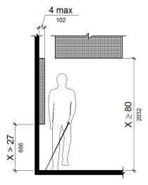
Figure 11B-307.2 Limits of Protruding Objects
