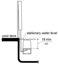
Figure 11B-1009.2.8 Pool Lift Submerged Depth
