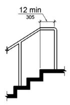
Figure *11B*-505.10.2 Top Handrail Extension at Stairs
