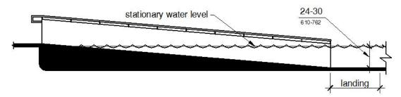
Figure 11B-1009.3.2 Sloped Entry Submerged Depth
