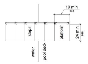
Figure 11B-1009.5.1 Size of Transfer Platform
