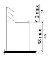
Figure 11B-904.3.2 Check-Out Aisle Counters
