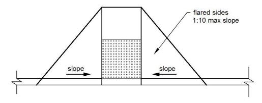
Figure 11B-406.2.2 Sides of Curb Ramps
