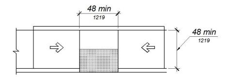
Figure 11B-406.3.2 Parallel Curb Ramps
