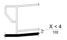
Figure 11B-405.9.2 Curb or Barrier Edge Protection
