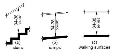
Figure 11B-505.4 Handrail Height
