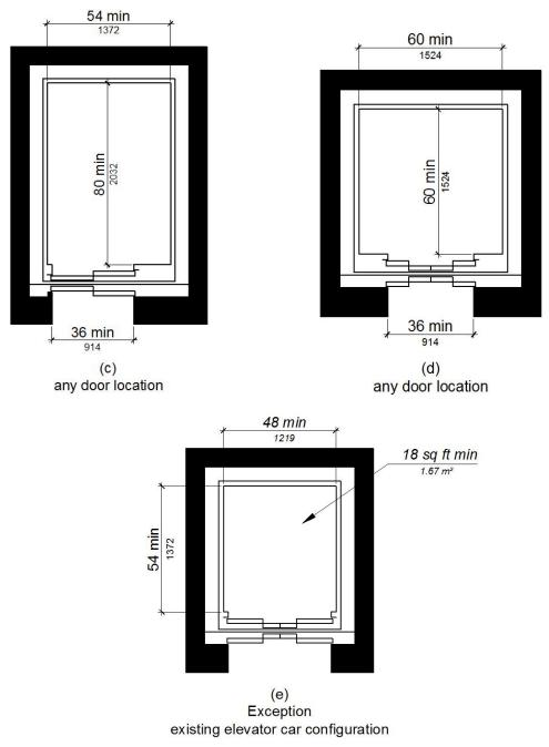
Figure 11B-407.4.1 Elevator Car Dimensions
