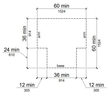
Figure 11B-304.3.2 T-Shaped Turning Space
