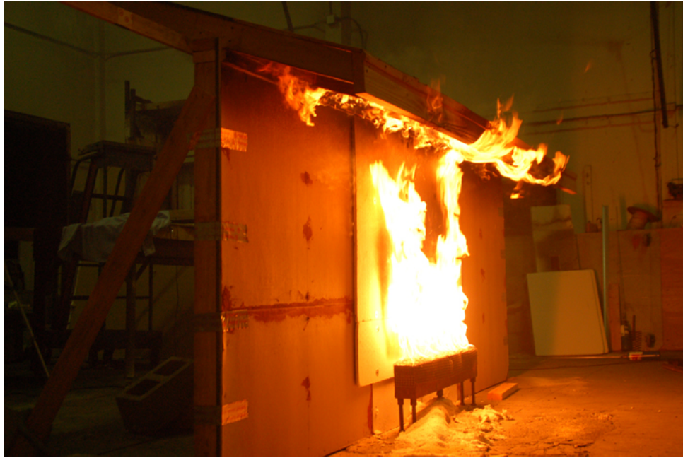
Figure 6. Lateral flame spread in the open-eave specimens usually spread to the end of the test wall within 30 to 60 s.
