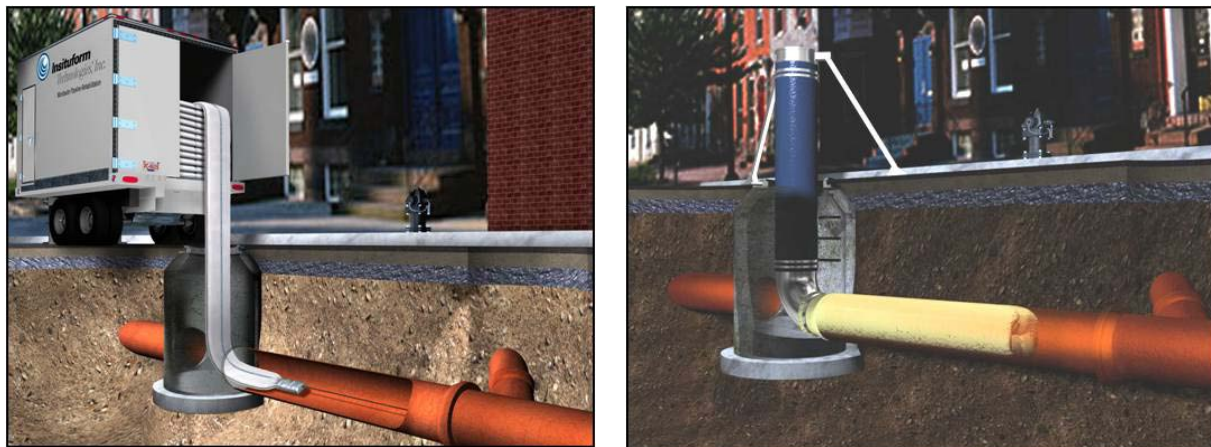
Figure 2-2. CIPP Installation Options: Liner Pull-in (Left) and Liner Inversion (Right) (Courtesy Insituform Technologies, Inc.)
