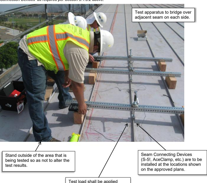
Test load shall be applied through the Seam Connecting Devices.
