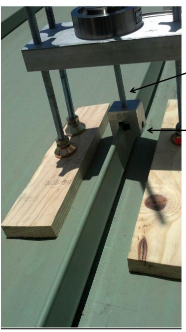
Test load shall be applied through the Seam Connecting Device
