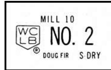
Figure 2-26: Visually Graded Framing Grade Stamp Example
