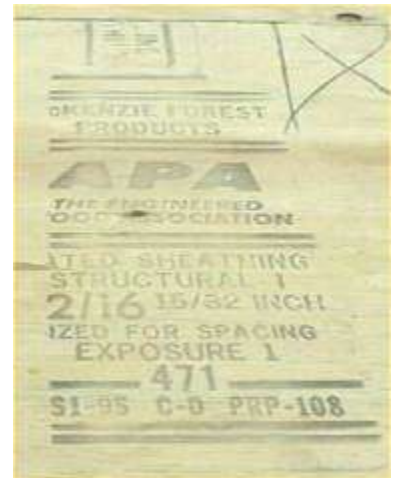
Figure 2-30: Example Wood Structural Panel Grade Stamp
