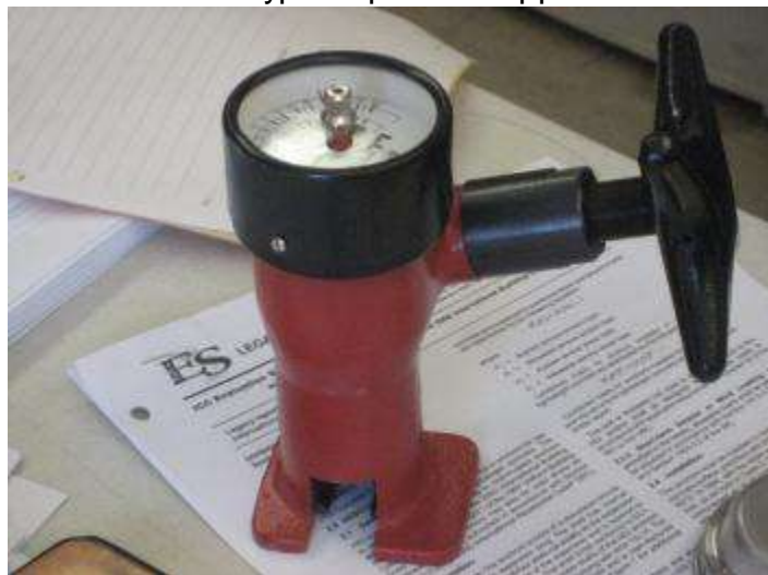
Figure 2-11: Example of a Common Pull Test Apparatus
