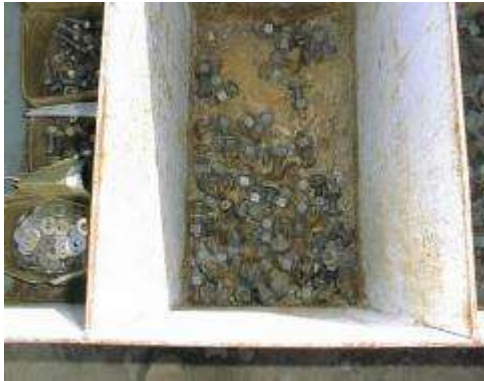
Figure 2-39: Improper HSB Storage
