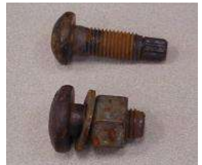
Figure 2-41: Twist-Off Type Tension Control Bolts
