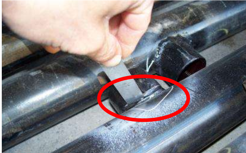
Figure 3-1: Rejected Sprinkler Pipe Due To Separation At Welds
