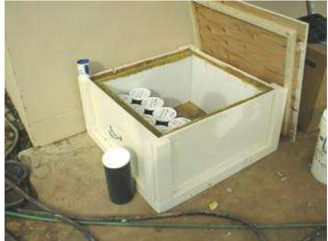
Figure 2-9: Proper Concrete Cylinder Storage
